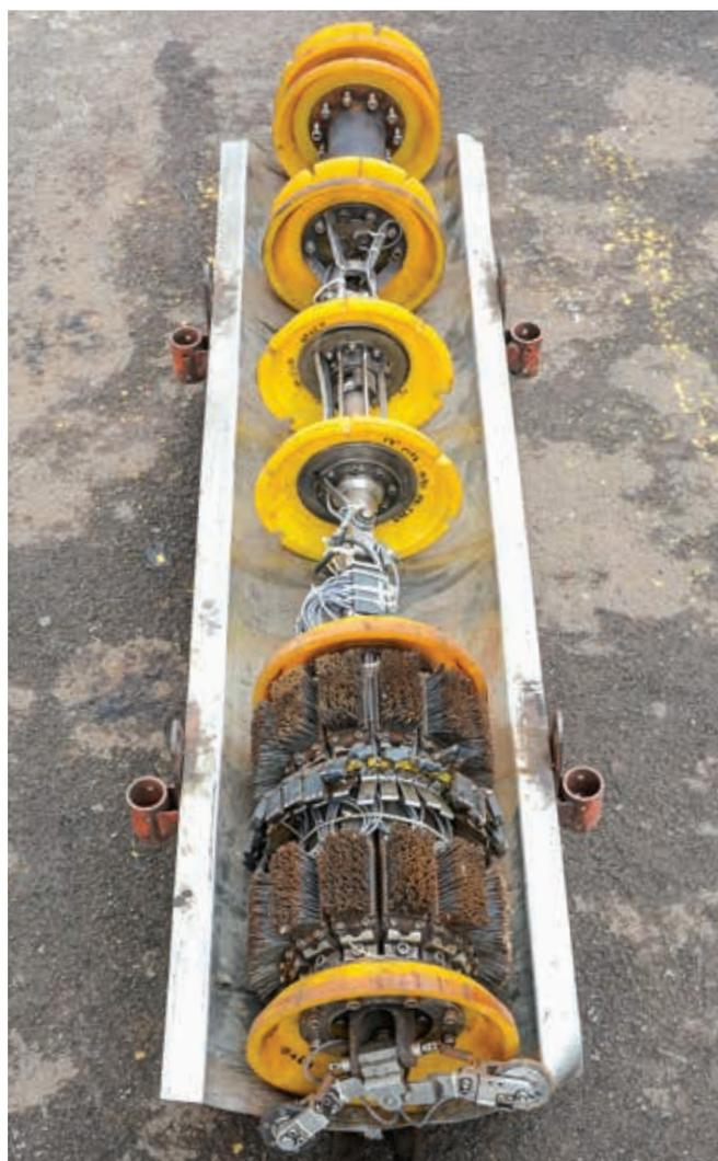
→ Pipeline Integrity check using Inspection Gauge
