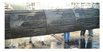
HPGRDC developed a novel cost effective Antifouling formulations by characterizing and studying the fouling deposits formed via various mechanisms in different refinery process heat exchangers.
