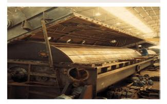
HPCL developed HP DWA V1 product to replace imported product in Propane dewaxing unit. Plant trials were successfully completed at Mumbai refinery and resulted in better performance with SPO and 150 N feed stock in terms of filtration. Due to good filtration, only two filters were taken inline vs 3 filters for reference additive. HPCL MR is extremely satisfied with the performance HPCL DWA V1 for 150N and SPO.
